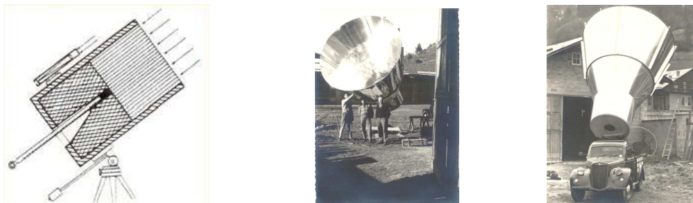
Fig. 5. Left: first honeycomb absorber that Francia built in 1960; Right: Photos of the first boiler coupled with a concentrator and protected by a honeycomb structure tested in Cesana Torinese in 1960/1961 (Francia Archive, Musil Brescia).
